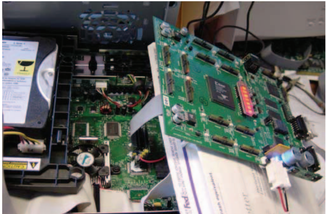
Figure 2. Andrew "bunnie" Huang's Xbox HyperTransport Bus tap circuit connecting an Xbox and FPGA development board (photo courtesy A. Huang).
